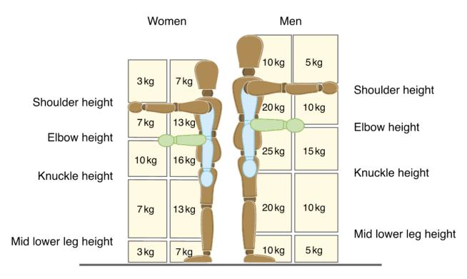
Figure 1 Lifting and lowering
